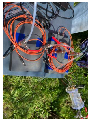
NETL sensors installed at an abandoned well, with 3D printed sensor assembly.
