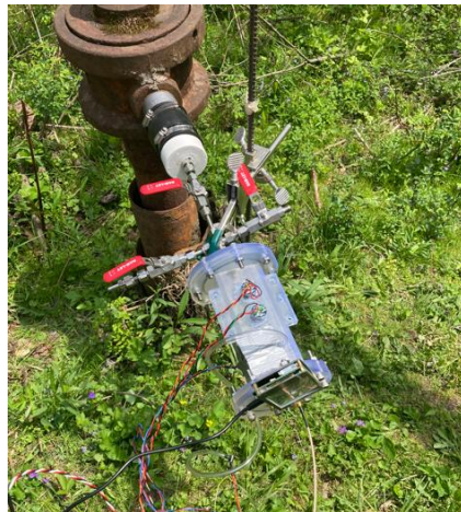
NETL sensors installed at an abandoned well, with 3D printed sensor assembly.
